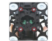
4.4 Install the Gimbal fixed block C-01, and tighten up it with four KM2x6 screws.
