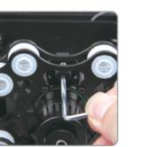
3.3 Fix the spring into M3x12 screw, then align the screw with the threaded hole and tighten to fix the Gimbal.
