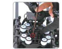
align the hole, and tighten the four M2x6 screws again, which below the screw column, then the installation completed.
