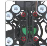
4.1 Loosen the four M2x6 screws above the Gimbal fixed block C-02, and take off the C-02.
